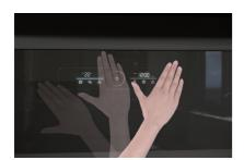
Motion sensors detect hand movements that pass through both sides of the control panel. The main unit can be turned on and off, and the air volume can be adjusted in large and small increments without the need for button operation.
